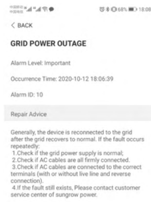
Figure 7-10 Detailed Fault Alarm Information
