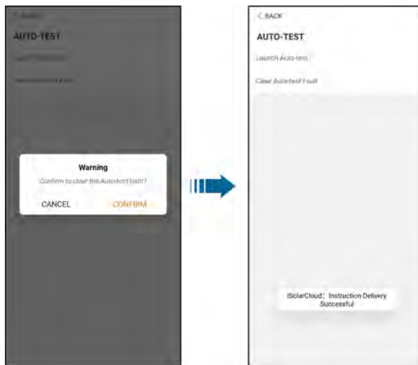
figure 7-23 Clear Auto-test Fault
