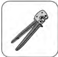
MC4 terminal crimping tool (4 mm 2 –6 mm 2 )
