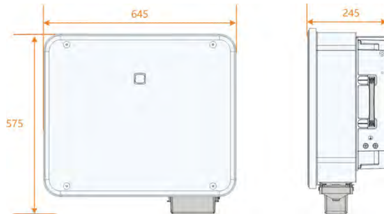
figure 2-3 Dimensions of the Inverter(in mm)
