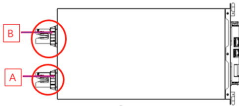
Figure1-4 Schematic diagram of the location of the no handling points A and B
