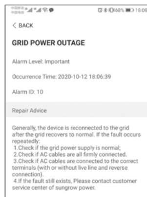
figure 7-9 Detailed Fault Alarm Information
