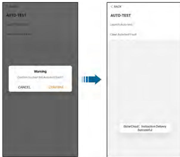
figure 7-25 Clear Auto-test Fault
