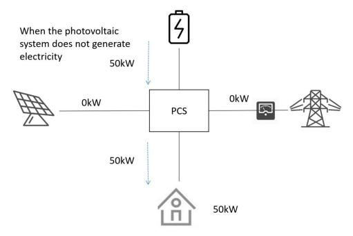
When PV power generation is insufficient to support the load, PV and energy storage jointly supply power to the load, as shown in the schematic diagram below:
