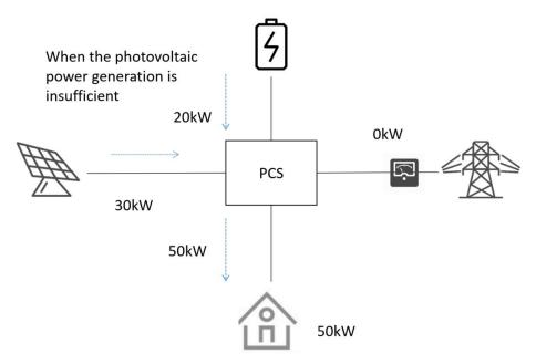
When neither PV nor battery power can support the load, the remaining power is taken from the grid, as shown in the schematic diagram below:
