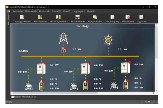
Method for replacing topology diagram file: Copy and replace the new topology diagram file "diagram. xml" to the SCADA program installation path C: \ AlphaESS \ AlphaCS-SCADA-FS Monitor \ project folder, and click the topology diagram button again to display the new topology diagram.
